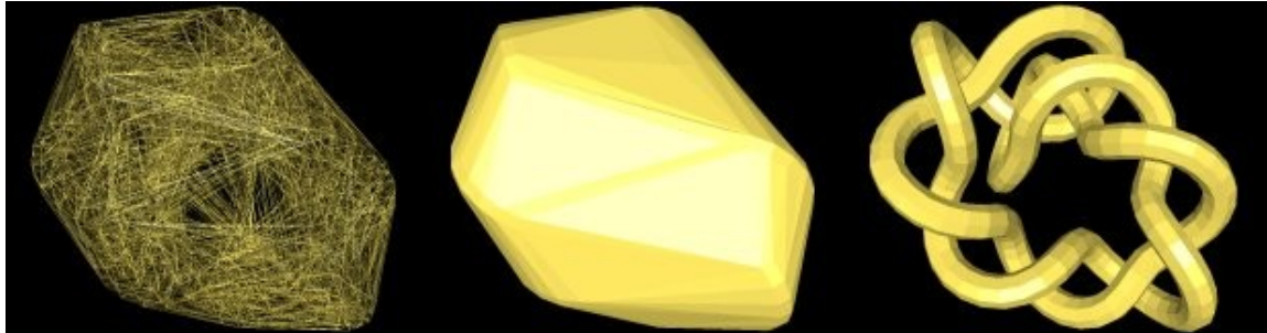
Figure 5: Wireframe (left) and solid (middle) representation of a Delaunay triangulation. Right: The corresponding surface.
